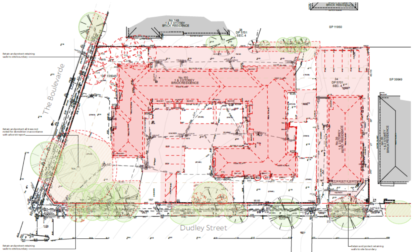
Figure 12 Detailed demolition plan (Source – Collins and Turner)
